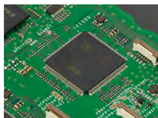
For band scope ADSP-21363 clock @332MHz
